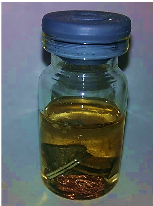
Figure 1. The process of dissolving lead in sulfuric acid.
